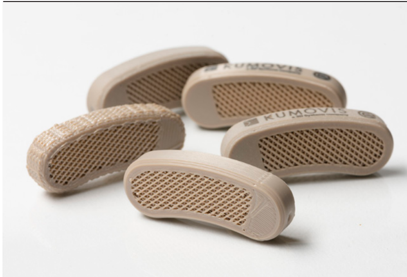
Figure 3 Sample for TLIF cage with porous structure and increased surface roughness.
