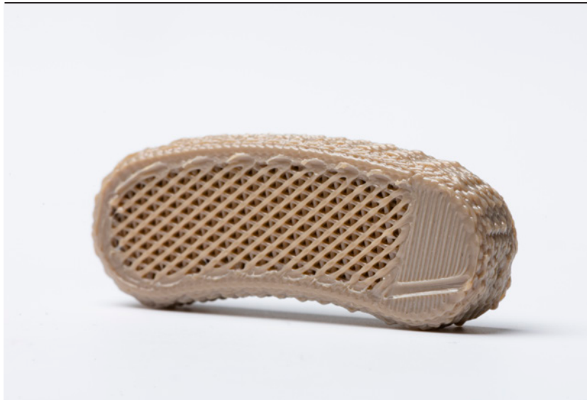
Figure 1 Case study design for TLIF spinal cage with porous infill made from VESTA- KEEP® Fusion.
